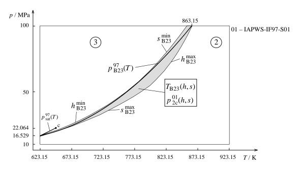
**Figure 5.** Illustration of the B23-equation  $p_{B23}^{97}(T)$  of IAPWS-IF97 and the range of validity of the boundary equation  $T_{B23}(h,s)$  in a p-T diagram
