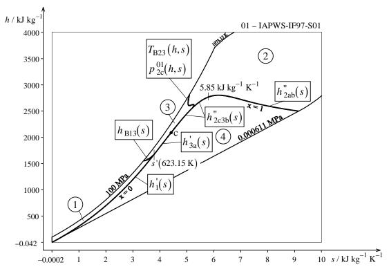
**Figure 3.** Regions of IAPWS-IF97 and boundary equations  $h_1(s)$ ,  $h_{3a}(s)$ ,  $h_{2ab}(s)$ ,  $h_{2c3b}(s)$ ,  $h_{B13}(s)$ , and  $T_{B23}(h,s)$  of this release
